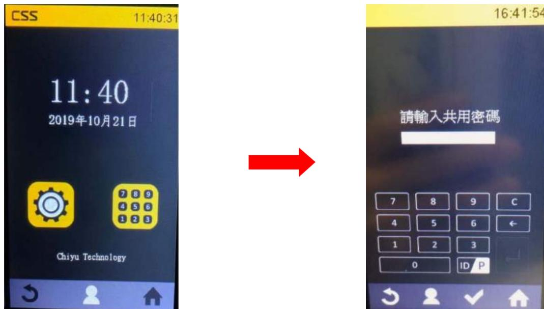
Personal password verification: Click on keypad icon → enter user ID and confirm by V → enter password and confirm by V, as shown below:
