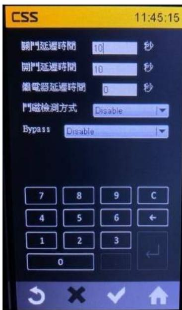
1. Door open delay time: Set the power open relay time, the factory default value is 10 seconds, can be set from 0 to 255 seconds.
